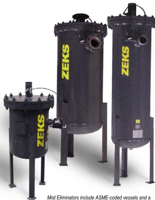
Mist Eliminators include ASME-coded vessels and a deep filter bed of special glass fibers packed between two layers of carbon steel screen.
